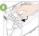
Fully tighten yoke T-handle clockwise.
