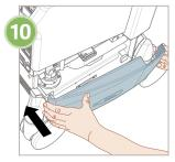
Slide helium tank drawer in and replace helium tank panel.
