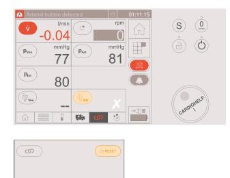
**20** Set the speed to 4000 rpm for 1 minute and then reduce speed to 0 rpm. De-air the 3 Luer lock connectors. If a bubble is detected, go back to step 18.
