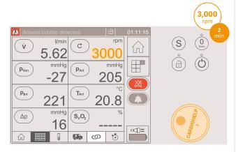
**19** Reduce speed to 0 rpm for at least 5 seconds. Reset the flow/bubble sensor. Tap the tube and the HLS Module with your hand to remove gas bubbles.
