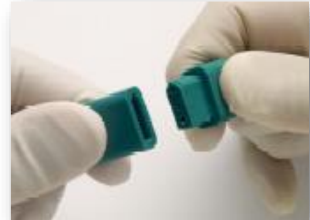
Match the triangular ends of the extension cable when connecting
